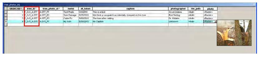
This is a view of the 'image' database called *tree\_photos\_ms*. Each entry is linked to a particular tree by the *Tree\_ID field*. There may be multiple entries for each tree. The database can be sorted like an excel database and the images are contained within this table.
